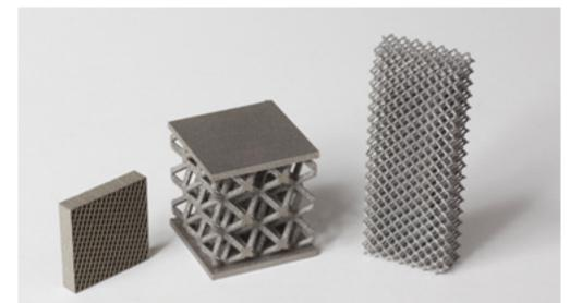
The **DMLS** (**Direct Metal Laser Sintering**) additive layer manufacturing (ALM) process produces metal components direct from a CAD model using a powerful 200w Yb-fibre laser to sinter or melt layers of fine metal powder together.
